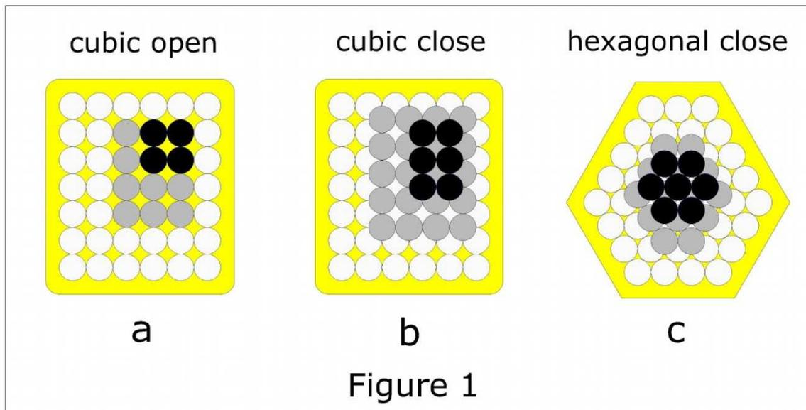
shown as Figure 1b. The "hexagonal close" depicted in Figure 1c, which is the dense packing adopted herein, is formed of triangular arrays nesting in the troughs beneath. Particles in the loosest arrangement touch 6 neighbouring spheres, the cubic close 8, and the hexagonal close 12.
