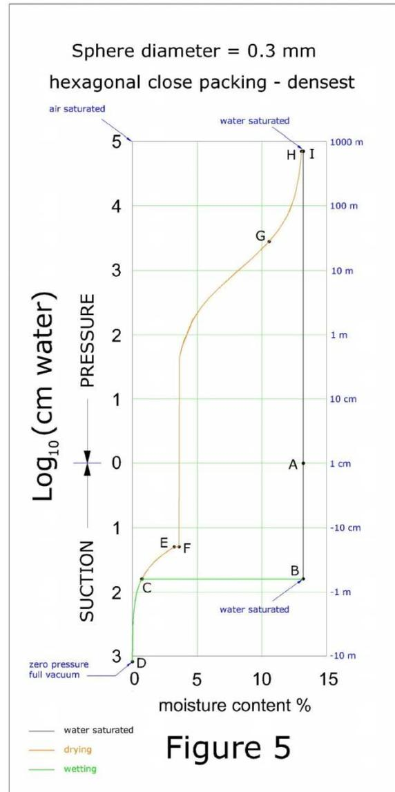
Point **I** is attained as a result of the air venting once **H** has been reached, thereby completing the wetting cycle and the soil becoming a water saturated 2-phase material again. This system cannot become air-entrained again without being subjected to the conditions attending Point **B**, and thereafter starting into another drying cycle.
