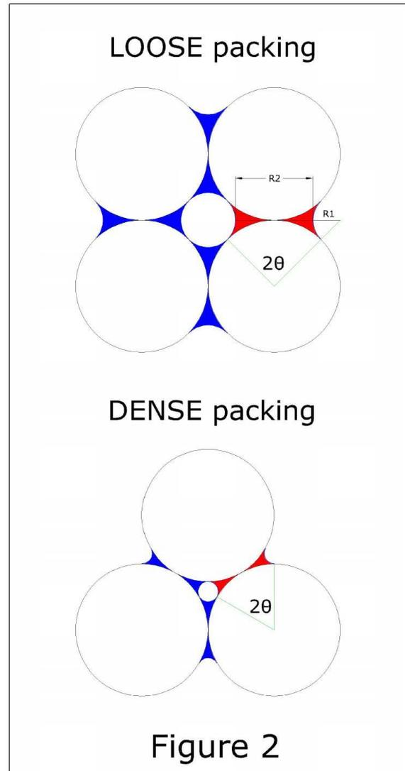
From the geotechnical point of view it is the surface tension force ( $T$ ) which is of primary interest since it dictates the pressure difference between the liquid and vapour phases. The following set of equations allow calculation of the pressure deficiency ( $PD$ ) between the water droplet with respect to the void air:
